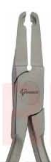
Pi6-71 Groove thermal forming plier Designed for making grooves on clear appliances, to hold the elastic, prevent it falling off
